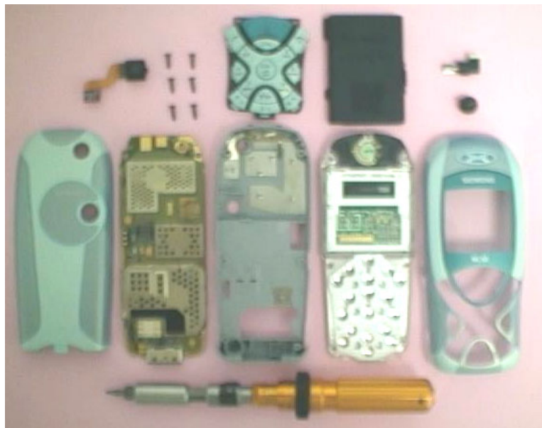
Fully disassembled MC 60
